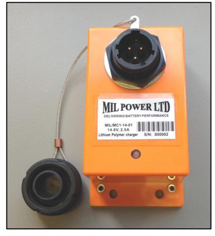
On connecting the battery to the charger the appropriate charge is applied automatically. Constant current or constant voltage is applied as required by the state of charge of the battery.
